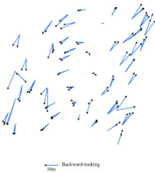
Fig. 5 Residuals of image observation (adjustment of principal positions)
